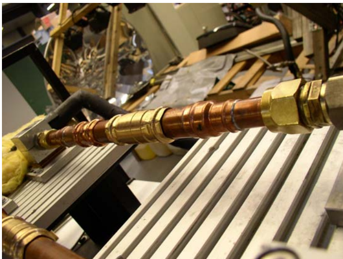
Figure 2: (before test start) Detail of installed test samples before testing.
